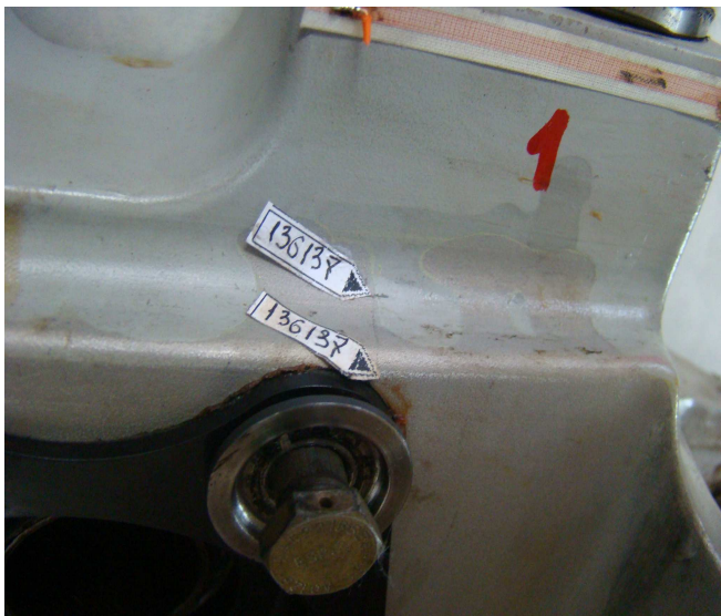
Fig.4 Fatigue crack of 15 mm length after 136137 loading cycle.
